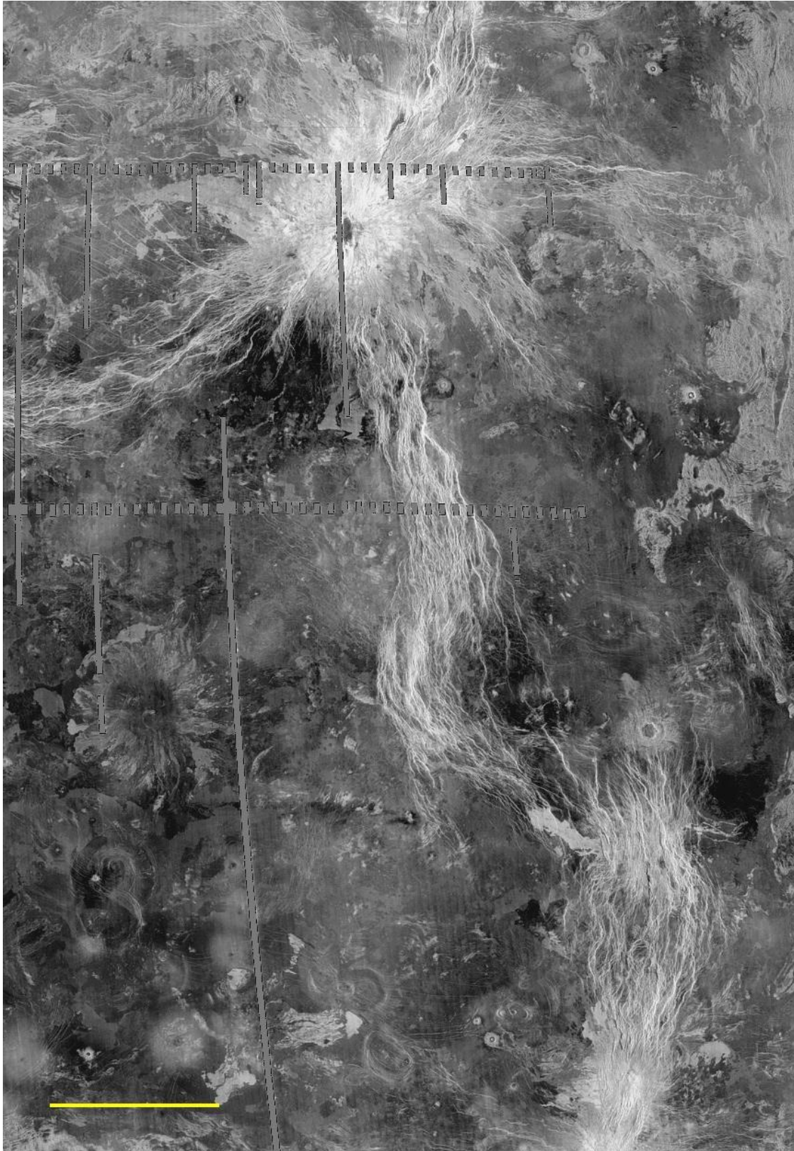
Figure 2.2. Magellan Radar Image of the Devana Chasma rift system, scale bar is 500 km. Note that the crater labeled A has been cut by the rift, with part of the crater visible on both sides of the rift. The thin linear features in the southern portion of this image are faults and fractures.
